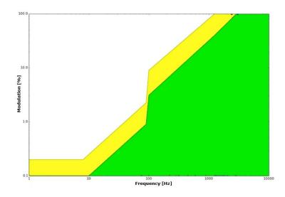
Thanks to its 4kHz dimming frequency, the LINE-5CV-CASAMBI effectively reduces the occurrence of the Flicker phenomenon. Depending on an individual's sensitivity and the nature of their activities, flickering can impact one's well-being, even if the changes in luminance are beyond the threshold detectable by the human eye.
